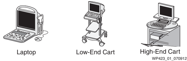
Figure 1: Scaling Down Ultrasound for Portability
