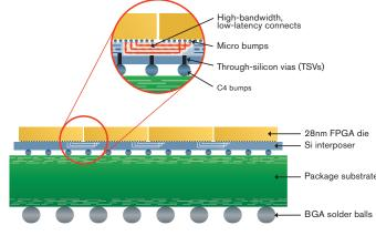
Figure 2. Schematic of package configuration
