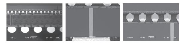
Figure 1. Cross-sections of (a) overall assembly, (b) TSV interposer, and (c) µbumps
